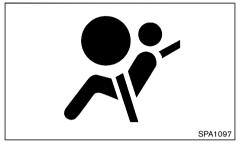
The supplemental air bag warning light, displaying in the instrument panel, monitors the circuits for the air bag systems, pre-tensioners and all related wiring.
