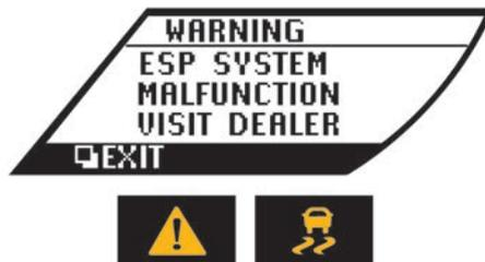
This will appear if the Electronic Stability Program (ESP) system or the hill start assist system is not functioning properly. (
