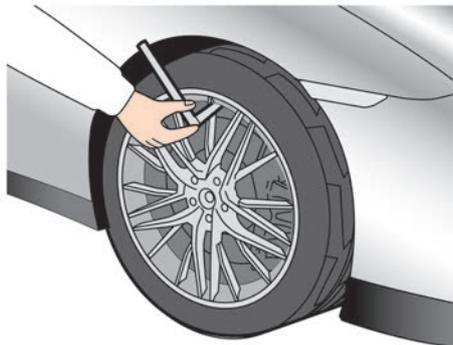
1. Remove the valve stem cap from the tire.
