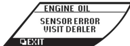
If the message shown above is displayed, the engine oil level sensor may be malfunctioning.
