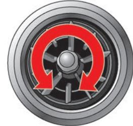
Turning the center knob clockwise or counterclockwise will close or open the ventilators.
