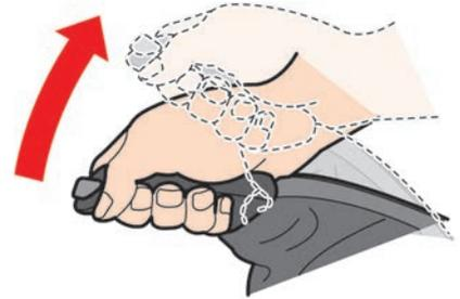
From the released position, pull the parking brake lever slowly and firmly. If the number of clicks is out of the range listed, see a NISSAN High Performance Center (NHPC).
