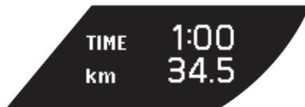
This displays the elapsed time and trip odometer beginning from the time when the display was last reset.
