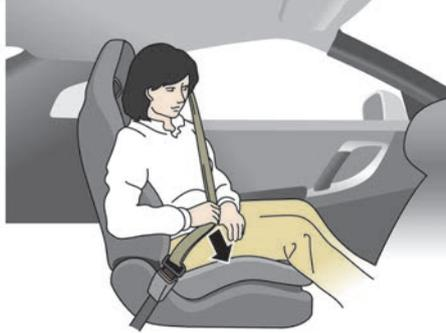
3. Position the lap belt portion **low and snug on the hips** as shown.
