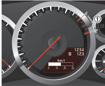
The tachometer indicates the engine speed in revolutions per minute (rpm). Do not rev the engine into the red zone ①.
