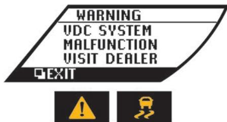
This will appear if the Vehicle Dynamic Control (VDC) system or the hill start assist system is not functioning properly. (
