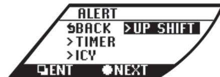
This function can be used to make settings for the upshift indicator, "timer" indicator and low outside temperature warning.
