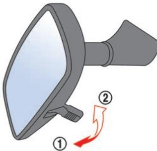
Pull the adjusting lever ① when the glare from the headlights of the vehicle behind you obstructs your vision at night.
