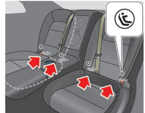
Your vehicle is designed to accommodate a child restraint system on the rear outer seats. Two ISOFIX anchoring points (located between the seat cushion and the seatback) are mounted directly on the body of the vehicle ensuring secure and stable attachment of the child restraint system.
