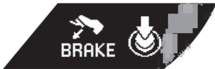
This indicator appears when the shift lever is in the **P** position.
