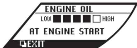
This can be used to check the pre-start oil level while the engine is running. Select SETTING > MAINTENANCE > OIL > ENGINE OIL > LEVEL.
