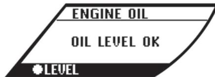
When the ignition switch is pushed to the ON position, the engine oil status before starting the engine is indicated as illustrated.
