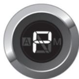
The transmission position indicator indicates the gear positions.
