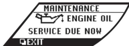
When the set mileage approaches, the reminder will appear on the display and the remaining distance is displayed at regular intervals. Select SETTING > MAINTENANCE > OIL > ENGINE OIL to set or reset the mileage for the engine oil change.
