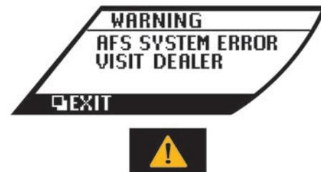
This will appear if the Adaptive Front Lighting System (AFS) is not functioning properly. Have the system checked by a NISSAN High Performance Center (NHPC). (
