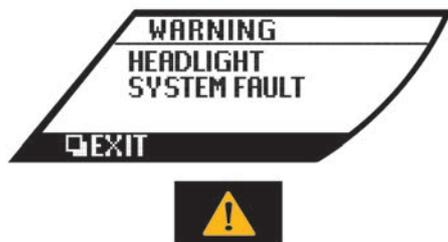
This will appear if the LED headlight system is not functioning properly. Have the system checked by a NISSAN High Performance Center (NHPC).
