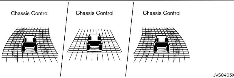
When the Intelligent Trace Control is operated and the "Chassis Control" mode is selected in the trip computer, the Intelligent Trace Control graphics are shown in the vehicle information display. (See "Trip computer" (P.2-41).)
