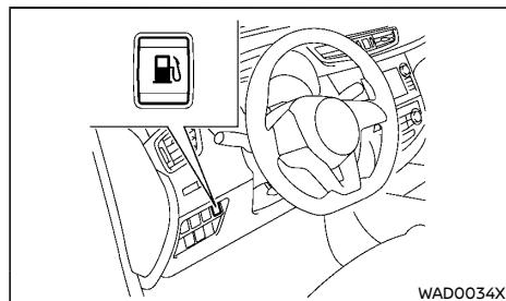
The fuel-filler lid opener switch is located on the instrument panel. To open, push the fuel-filler lid opener switch. To lock, close the fuel-filler lid securely.
