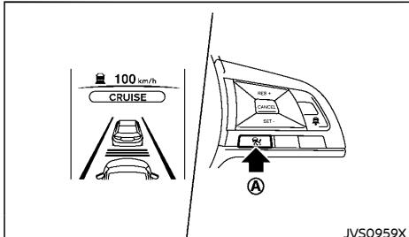
**To turn on the cruise control,** quickly push and release the CRUISE ON/OFF switch Ⓐ. The ICC system ON indicator (gray), set distance indi-
