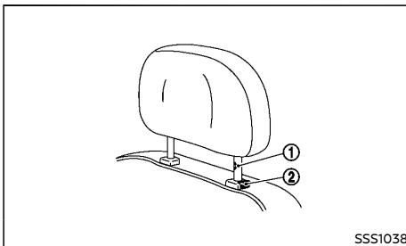
1. Align the head restraint stalks with the holes in the seat. Make sure that the head restraint is facing the correct direction. The stalk with the adjustment notch ① must be installed in the hole with the lock knob ②.
