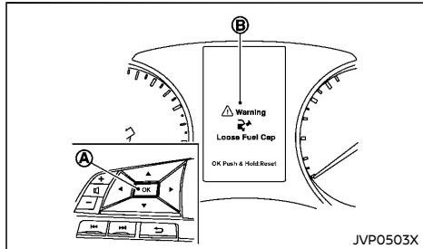
The LOOSE FUEL CAP warning message is displayed on the vehicle information display when the fuel-filler cap is not tightened correctly after the vehicle has been refueled. It may take a few driving trips for the message to be displayed.
