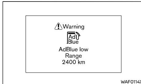
This warning appears when the AdBlue® level in the tank is getting low. The message will be displayed each time the engine starts when there is estimated to be between 2,400 and 800 km (1,500 and 500 miles) left before the AdBlue® tank becomes empty. The message can be cleared from the display until the next time the engine is started.
