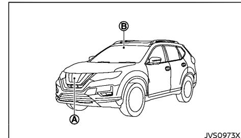
The Intelligent Emergency Braking with pedestrian detection system uses a radar sensor **A** located on the front of the vehicle to measure
