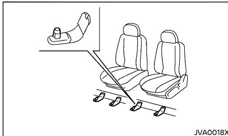
This vehicle includes front floor mat brackets to act as a floor mat positioning aid. NISSAN floor mats have been specially designed for your vehicle model.
