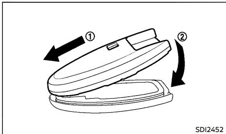
4. Align the tips of the upper and lower parts ①, and then push them together until it is securely closed ②.
