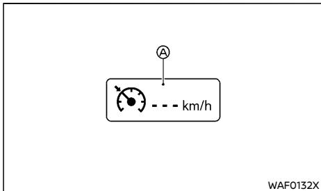
When pushing the ICC ON/OFF switch ④ on, the conventional (fixed speed) cruise control mode display and indicators ④ are displayed in the vehicle information display. After you hold the ICC ON/OFF switch for longer than about 1.5 seconds, the ICC system display goes out. The cruise indicator appears. You can now set your desired cruising speed. Pushing the ICC ON/OFF switch again will turn the system completely off.
