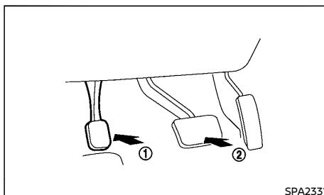
To apply the parking brake, firmly depress the parking brake pedal ①.
