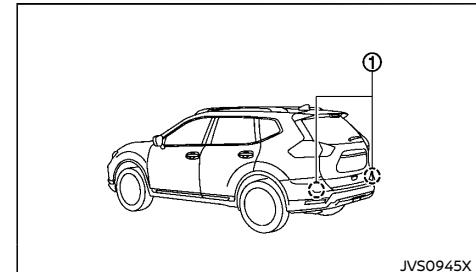
The two radar sensors ① for the BSW system are located near the rear bumper. Always keep the area near the radar sensors clean.
