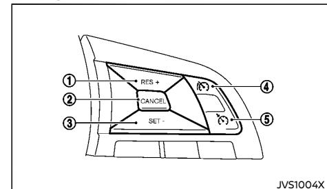
The speed limiter set switches are located on the steering wheel.
