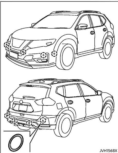
Parking sensors (sonar) are located on the bumpers: 6 on the front bumper and 4 on the rear bumper.
