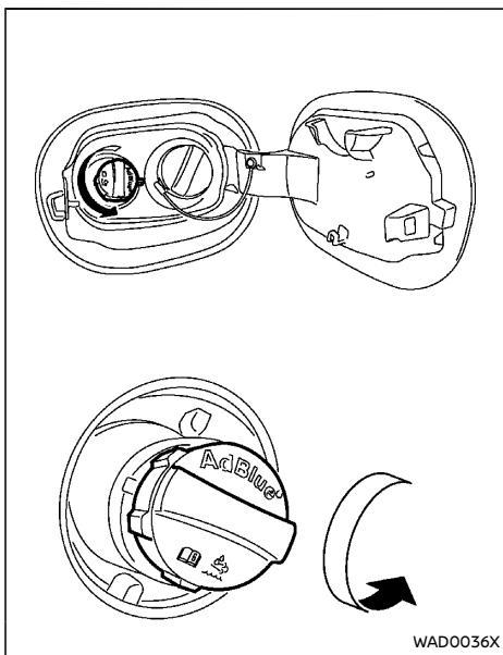
Turn the cap counterclockwise to remove.
