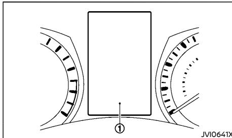
The vehicle information display ① is located between the tachometer and the speedometer. It displays following items if the vehicle is equipped with them:
