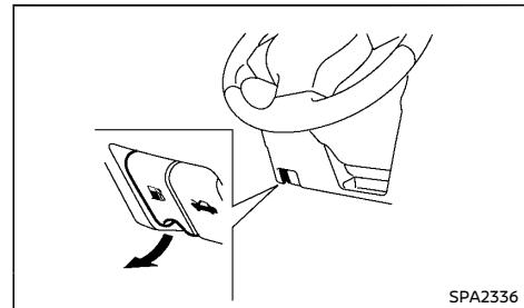
To open the AdBlue® filler lid, pull the fuel-filler lid release handle.
