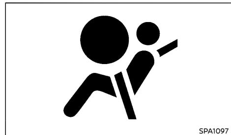
The SRS air bag warning light, displaying in the meter, monitors the circuits for the air bag systems, pre-tensioner seat belt systems and all related wiring.
