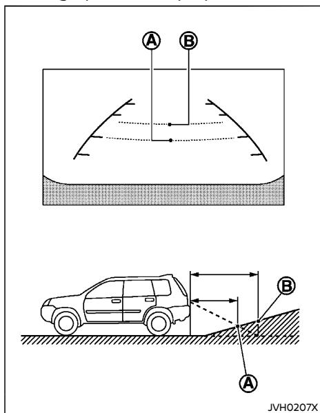
When backing up the vehicle up a hill, the distance guide lines and the vehicle width guide lines are shown closer than the actual distance. For example, the display shows 1 m (3 ft) to the place Ⓐ, but the actual 1 m (3 ft)
