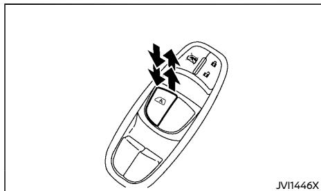
The automatic function is available for the switch that has an **A** mark on its surface.
