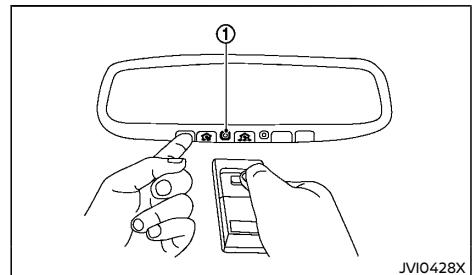
2. Using both hands, simultaneously press and hold the desired HomeLink® button and handheld transmitter button. DO NOT release until the HomeLink® indicator light ① flashes slowly and then rapidly. When the indicator light flashes rapidly, both buttons may be released. (The rapid flashing indicates successful programming.)
