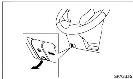
To open the fuel-filler lid, pull the fuel-filler lid release handle.
