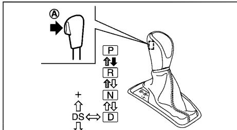
CVT with manual shift mode (Type B) or DCT (LHD model)
