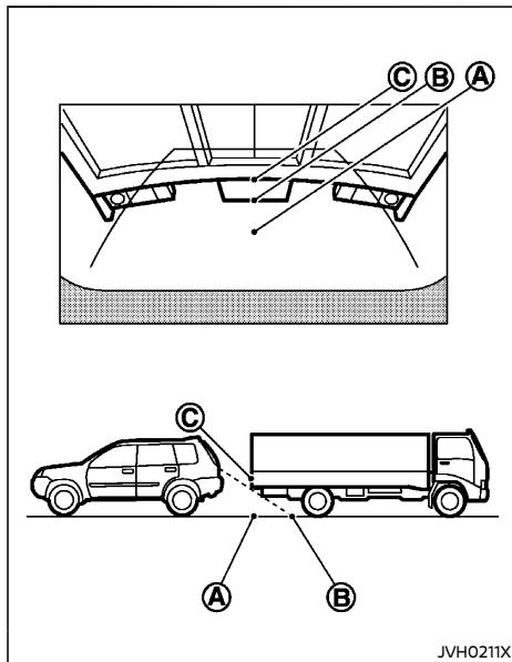
The position © is shown further than the position ® in the display. However, the position © is actually at the same distance as the position ®. The vehicle may hit the object when backing up to the position ® if the object projects over the actual moving course.
