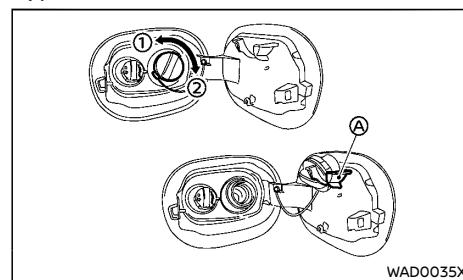
The fuel-filler cap is a ratcheting type. Turn the cap counterclockwise ① to remove. Tighten the cap clockwise ② until ratchet clicks, more than twice, after refueling.
