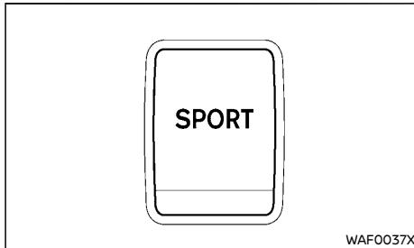
The SPORT mode switch adjusts the engine and transmission points to enhance performance. Push the SPORT mode switch on the instrument panel to activate. The SPORT mode indicator appears in the vehicle information display.
