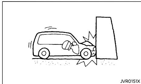
The supplemental front-impact air bag system will deploy in the event of an impact which exceeds a 25 km/h (16 MPH) frontal collision with a solid wall that does not move or deform.
