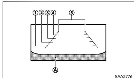
Guiding lines which indicate the vehicle width
