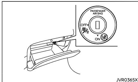
The front passenger air bag can be turned off with the front passenger air bag switch located in the glove box.
