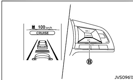
**To set cruising speed,** accelerate your vehicle to the desired speed, push the SET/- switch Ⓐ and release it. (The ICC system set indicator (green), vehicle ahead detection indicator, set distance indicator and set vehicle speed indicator come on.) Take your foot off the accelerator pedal. Your vehicle will maintain the set speed.
