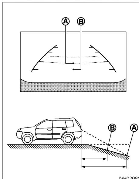
When backing up the vehicle down a hill, the distance guide lines and the vehicle width guide lines are shown further than the actual distance. For example, the display shows 1 m (3 ft) to the place Ⓑ, but the actual 1 m (3 ft)
