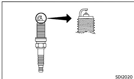
It is not necessary to replace the iridium-tipped spark plugs as frequently as the conventional type of spark plugs. These spark plugs are designed to last much longer than the conventional type of spark plug.
