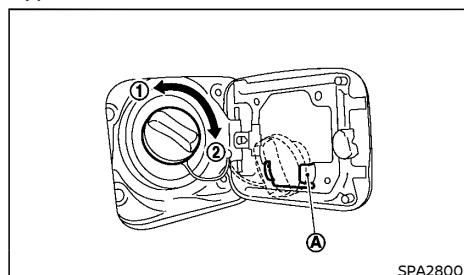
Put the fuel-filler cap on the cap holder Ⓐ while refueling.
