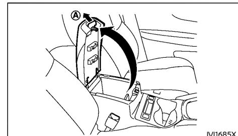
To open the console box lid, push up the knob Ⓐ and pull up the lid.
