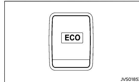
The ECO mode system helps to enhance the fuel economy by controlling the engine and CVT/DCT operation automatically to avoid rapid acceleration.
