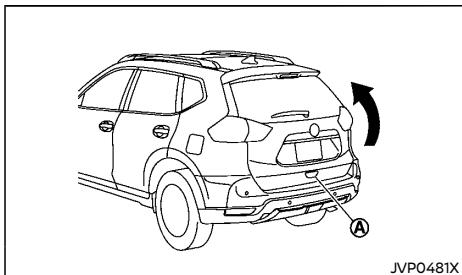
To open the back door, unlock it and push the opener switch ①. Pull up the back door to open. The back door can be unlocked by:
