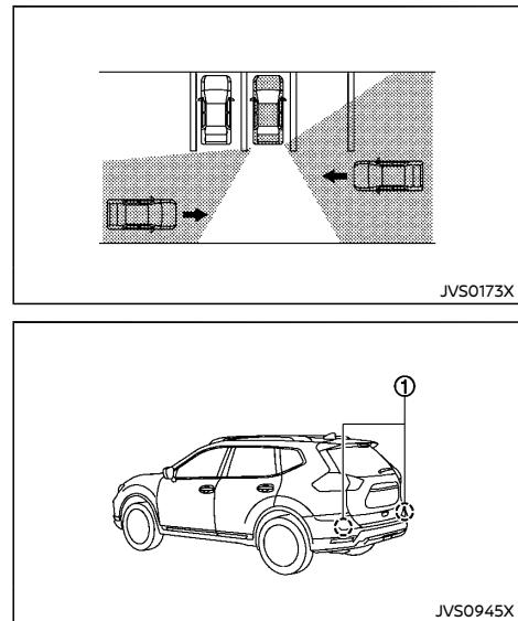
The RCTA system uses radar sensors ① installed on both sides near the rear bumper to detect an approaching vehicle.
