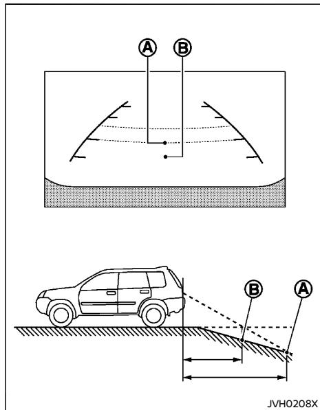
When backing up the vehicle down a hill, the distance guide lines and the vehicle width guide lines are shown further than the actual distance. For example, the display shows 1 m (3 ft) to the place Ⓐ, but the actual 1 m (3 ft) distance on the hill is the place Ⓑ. Note that any object on the hill is closer than it appears on the monitor.
