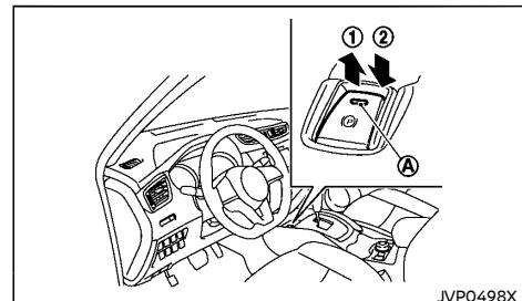
The electronic parking brake can be applied or released automatically or by operating the parking brake switch.
