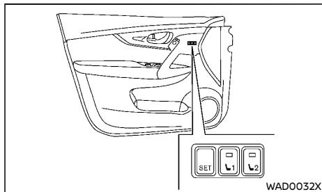
Two positions for the driver's seat and outside mirrors can be stored in the automatic drive positioner memory. Follow these procedures to use the memory system.
