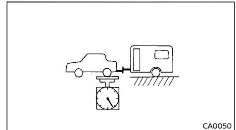
The rear gross axle weight must not exceed the Gross Axle Weight Rating (GAWR).
