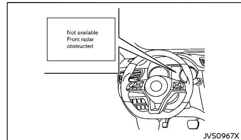
The chime will sound and the "Not available: Front radar obstructed" warning message will appear in the vehicle information display.
