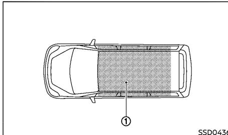
The Intelligent Key can only be used for starting the engine when the Intelligent Key is within the specified operating range ①.
