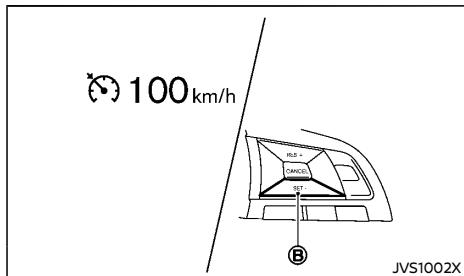
**To set cruising speed**, accelerate your vehicle to the desired speed, push the SET/- switch ⑧ and release it. (The color of the cruise indicator changes to green and set vehicle speed indicator comes on.) Take your foot off the accelerator pedal. Your vehicle will maintain the set speed.
