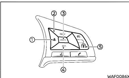
1. Push the ProPILOT switch (5). This turns on the ProPILOT system and displays the status of the ProPILOT system on the
