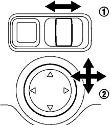
The outside rearview mirror remote control operates when the ignition switch is in the "ACC" or "ON" position.
