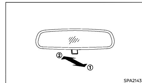
Pull the adjusting lever ① when the glare from the headlights of the vehicle behind you obstructs your vision at night.
