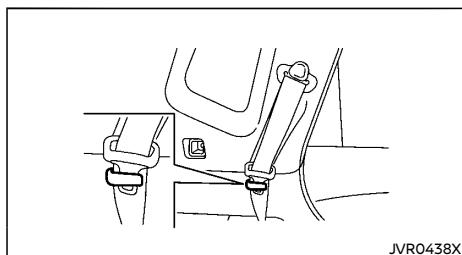
Seat belt can be hooked on the belt hook.
