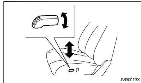
Pull up or push down the adjusting switch to adjust the seat height until the desired position is achieved.
