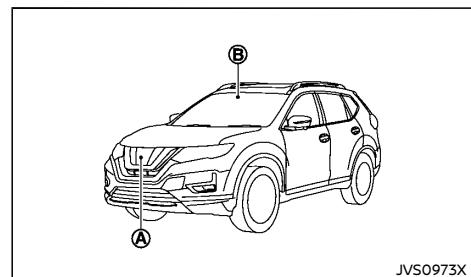
The radar sensor **A** is located on the front of the vehicle. The camera **B** is located on the upper side of the windshield.
