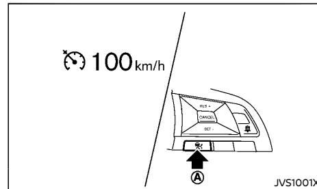
To turn on the conventional (fixed speed) cruise control mode, push and hold the Cruise ON/OFF switch Ⓐ for longer than about 1.5 seconds.
