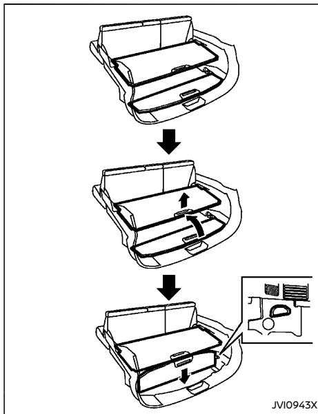
1. Place the inner board on the upper position. (See "Three-stage mode" (P.2-73).)
