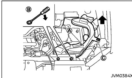
Remove the air duct and resonator (MR20DD engine) if necessary.
