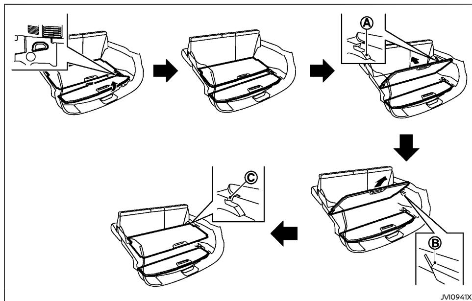
1. Pull the outer board upward to about 30°.
