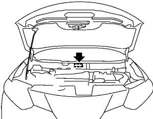
The vehicle identification number is located as shown.
