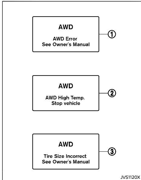
If the "AWD Error" warning ① appears, there may be a malfunction in the Intelligent 4x4 system. Reduce vehicle speed and have your vehicle checked by a NISSAN dealer as soon as possible.
