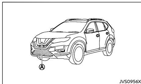
The sensor **A** is located on the front of the vehicle.
