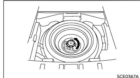
Remove the clamp holding the spare tire.
