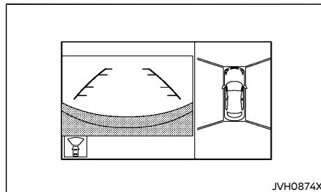
With the ignition switch in the "ON" position, push the CAMERA button (if equipped)/DISP button (if equipped) or move the shift lever to the "R" (Reverse) position to operate the Intelligent Around View Monitor/Around View Monitor.
