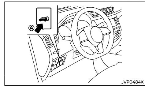
Power back door switch – Instrument panel JVP0484X
