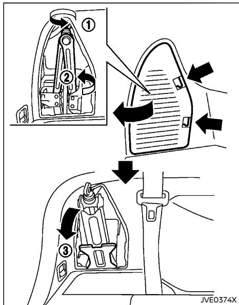
1. Remove the storage door by pressing the two release tabs simultaneously.
