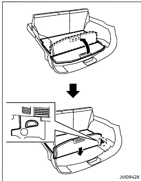
1. Pull the outer board upward to 90°.
