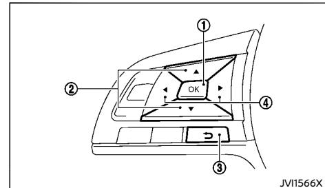
The vehicle information display can be changed using the buttons OK ①, ②, ③, and ④ located on the steering wheel.
