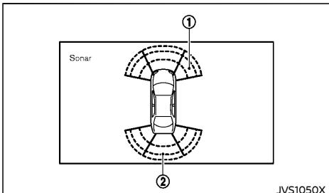
When the corner of the vehicle moves closer to an object, the parking sensor indicators ① appears (if equipped).
