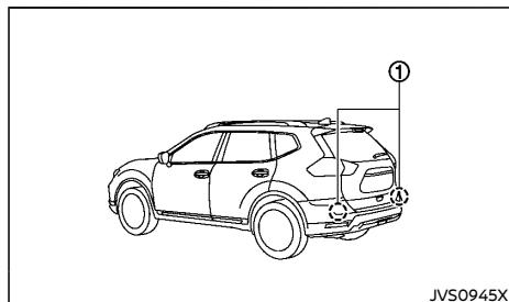
The two radar sensors ① for the RCTA systems are located near the rear bumper. Always keep the area near the radar sensors clean.
