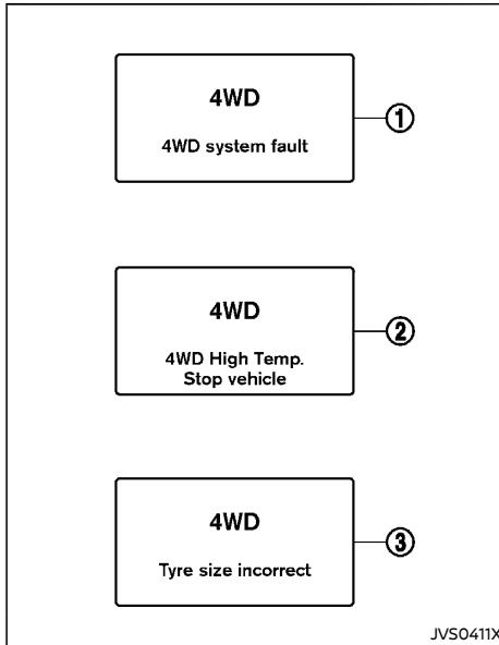
If the "4WD system fault" warning ① appears, there may be a malfunction in the 4WD system. Reduce vehicle speed and have your vehicle checked by a NISSAN dealer as soon as possible.
