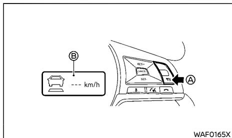
To turn the cruise control on, quickly push and release the ICC ON/OFF switch **A**. A Popup message is displayed showing ICC ON and steering assist status (when steering assist is turned on using the vehicle information display). The ICC system ON indicator (gray), and set vehicle speed indicator --- **B** come on.
