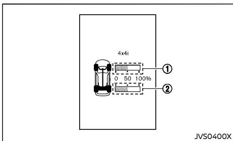
When the Intelligent 4x4 torque distribution display is selected, you can view the distribution ratio of the transmission torque to the front and rear wheels during driving. The Intelligent 4x4 torque distribution display is shown on the vehicle information display screen.
