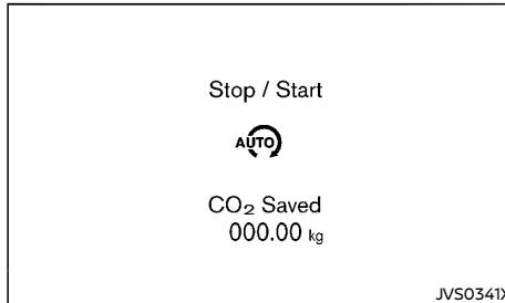
When the engine is stopped the information is displayed for a few seconds.
