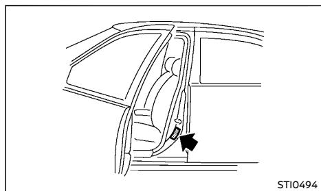
The cold tire pressures are shown on the tire placard affixed to the driver's side center pillar.
