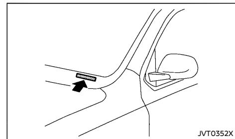
The vehicle identification number plate is attached as shown. This number is the identification for your vehicle and is used in the vehicle registration.
