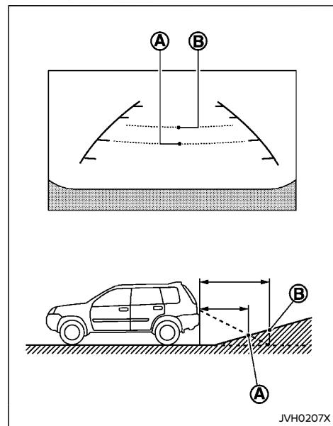
When backing up the vehicle up a hill, the distance guide lines and the vehicle width guide lines are shown closer than the actual distance. For example, the display shows 1 m (3 ft) to the place Ⓐ, but the actual 1 m (3 ft) distance on the hill is the place Ⓑ. Note that any object on the hill is further than it appears on the monitor.
