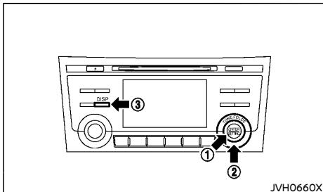
To set up the Intelligent Around View Monitor/Around View Monitor display to your preferred settings, push the ENTER/SETTING button ① while the Intelligent Around View Monitor/Around View Monitor screen is displayed. Each time the ENTER/SETTING button ① is pushed, the next setting item is selected. Turn the TUNE-FOLDER dial ② to adjust each item.
