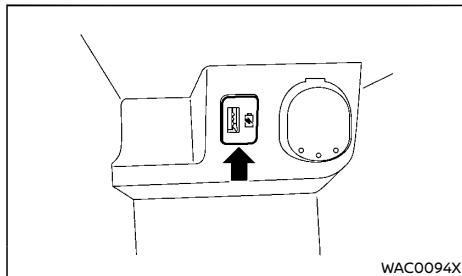
The USB charging connector is located in the center console box.
