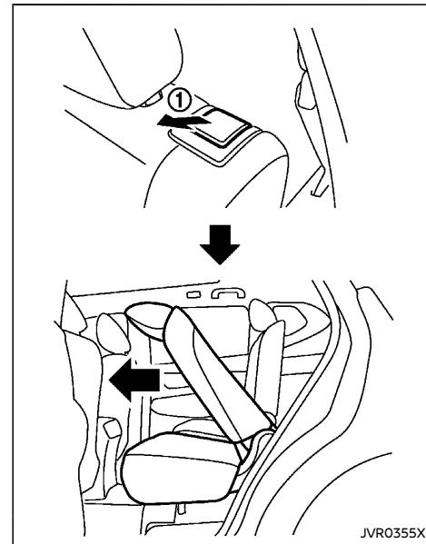
1. Pull the lever ① to tilt down the seatback.
