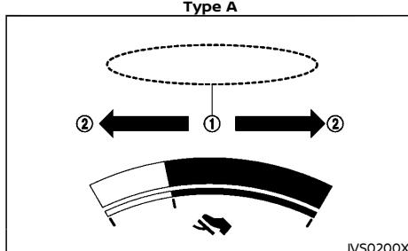
The ambient ECO ① is displayed according to the accelerator pedal operation, while driving the vehicle in ECO mode.
