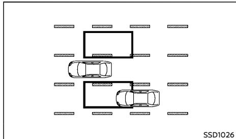
The Blind Spot Indicator light illuminates if a vehicle enters the detection zone from behind in an adjacent lane.
