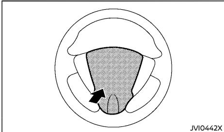
The horn switch
