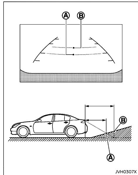
When moving the vehicle up a hill, the distance guide lines and the vehicle width guide lines are shown closer than the actual distance. For example, the display shows 1 m (3 ft) to the place ⑥, but the actual 1 m (3 ft) distance on the hill is the place ⑦. Note that any object on the hill is viewed in the monitor further than it appears.
