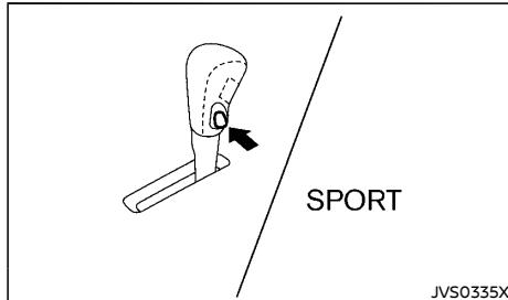
To select the SPORT mode, push the SPORT mode switch with the shift lever in the "D" (Drive) position. The SPORT mode indicator light **SPORT** in the meter panel illuminates. To turn off the SPORT mode, push the SPORT mode switch again. The SPORT mode indicator light will turn off. When the shift lever is shifted to any position other than "D" or "Ds", the SPORT mode will be automatically turned off.
