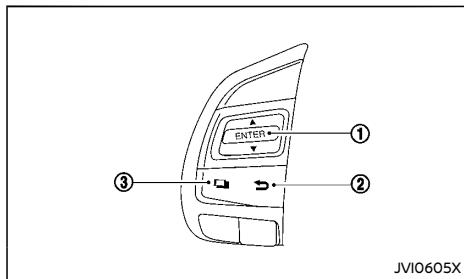
The vehicle information display can be changed using the switches ③ and ENTER ① located on the steering wheel.
