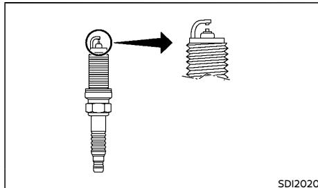
It is not necessary to replace the iridium-tipped spark plugs as frequently as the conventional type of spark plugs. These spark plugs are designed to last much longer than the conventional type of spark plug.
