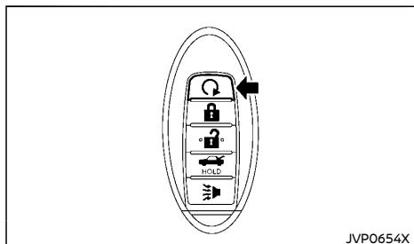
The remote engine start button is on the Intelligent Key if the vehicle has remote engine start function. This function allows the engine to start from outside the vehicle.
