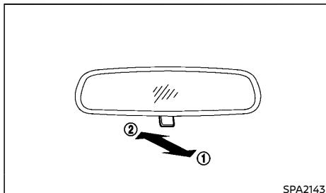
Pull the adjusting lever ① when the glare from
