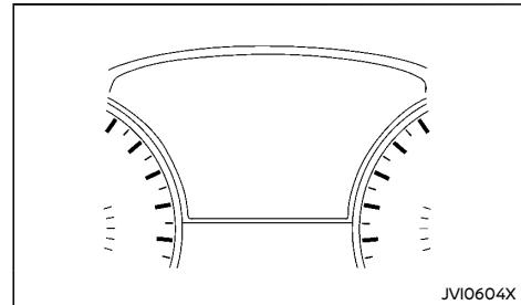
The vehicle information display is located on the left of the speedometer. It displays such items as:
