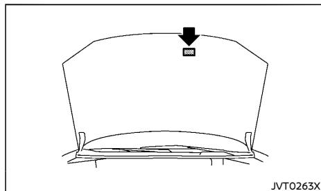
The air conditioner specification label is attached to the underside of the hood as shown.
