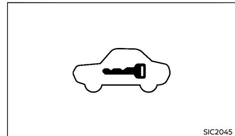
The security indicator light, located on the meter panel, operates whenever the ignition switch is in the "LOCK", "OFF" or "ACC" position. This is normal.
