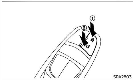
Operating the power door lock switch, located on the driver's door armrest, will lock or unlock all the doors.
