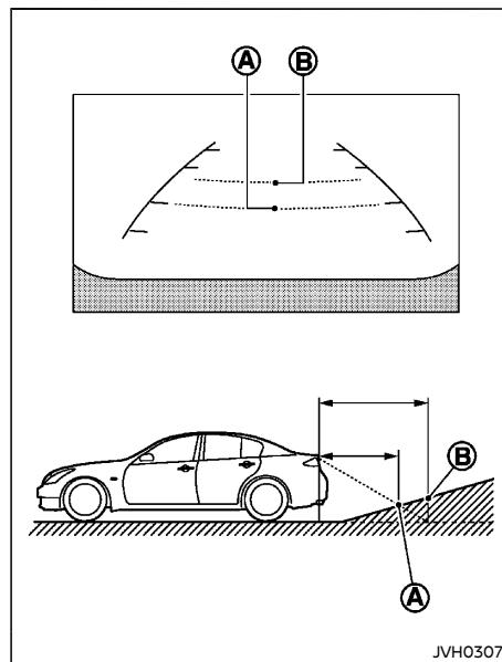
When moving the vehicle up a hill, the distance guide lines and the vehicle width guide lines are shown closer than the actual distance. For example, the display shows 1 m (3 ft) to the place Ⓐ, but the actual 1 m (3 ft) distance on the hill is the place Ⓑ. Note that any object on the hill is viewed in the monitor further than it appears.
