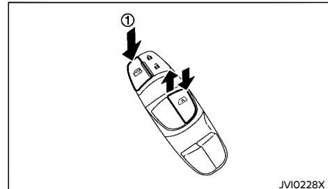
The driver's switch, the main switch, can control all windows.
