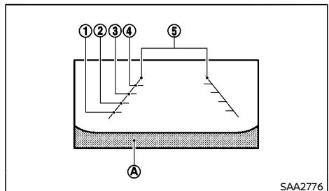
Guiding lines which indicate the vehicle width and distances to objects with reference to the bumper line ⑥ are displayed on the monitor.
