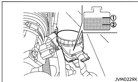
Check the fluid level in the reservoir. If the fluid is below the MIN line ②, the brake warning light will illuminate. Add fluid up to the MAX line ①. (See "Recommended fluids/lubricants and capacities" (P.9-2) for recommended types of fluid.)
