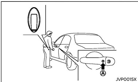
When you carry the Intelligent Key with you, you can lock or unlock all doors by pushing the door handle request switch Ⓐ within the range of operation.
