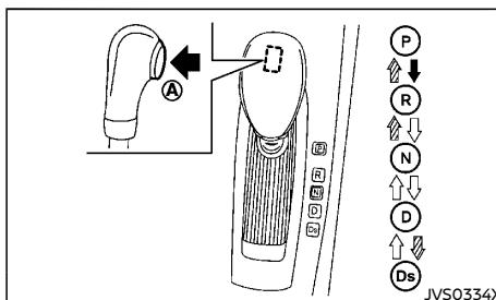
→ Push the button A while depressing the foot brake pedal.
