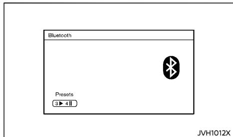
To switch to the Bluetooth® audio mode, push the USB-AUX button repeatedly until the Bluetooth® audio mode is displayed on the screen.
