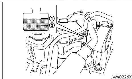
Check the coolant level in the reservoir tank when the engine is cold. If the coolant level is below the MIN level ②, add coolant up to the MAX level ①. If the reservoir tank is empty, check the coolant level in the radiator **when the engine is cold**. If there is insufficient coolant in the radiator, fill the radiator with coolant up to the filler opening and also add it to the reservoir tank up to the MAX level ①.
