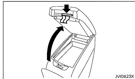
Pull up on the driver's side latch to open the upper half of the console box.
