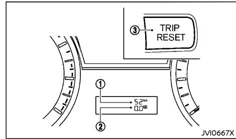
The odometer ① and the twin trip odometer ② are displayed below the vehicle information display when the ignition switch is placed in the "ON" position.
