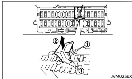
To reduce battery drain, the extended storage fuse switch comes from the factory switched off. Prior to delivery of your vehicle, the switch is pushed in (switched on) and should always remain on.
