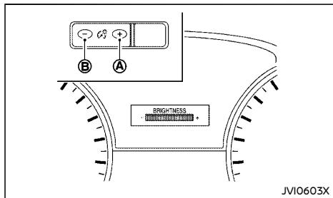
Push the "+" side **A** to increase the brightness of meter panel lights.
