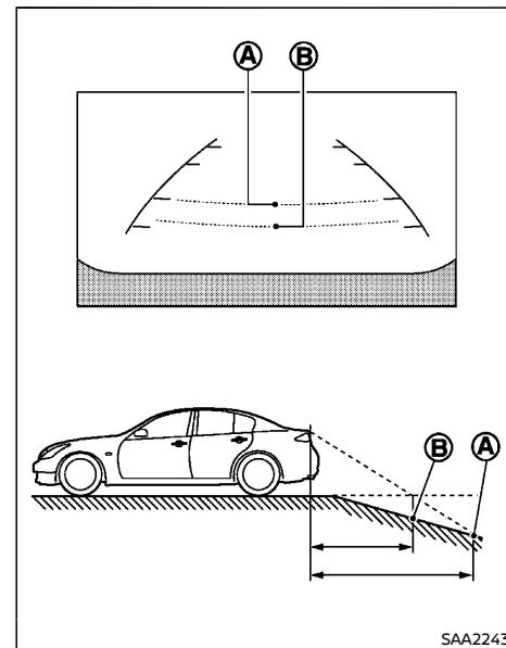
When moving the vehicle down a hill, the distance guide lines and the vehicle width guide lines are shown further than the actual distance. For example, the display shows 1 m (3 ft) to the place Ⓑ, but the actual 1 m (3 ft) distance on the hill is the place Ⓐ. Note that any object on the hill is viewed in the monitor closer than it appears.
