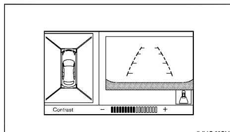
To set up the Intelligent Around View Monitor to your preferred settings, push the ENTER/SETTING button ① while the Intelligent Around View Monitor screen is displayed. Each time the ENTER/SETTING button ① is pushed, the next setting item is selected. Turn the TUNE-FOLDER control knob ② to adjust each item.
