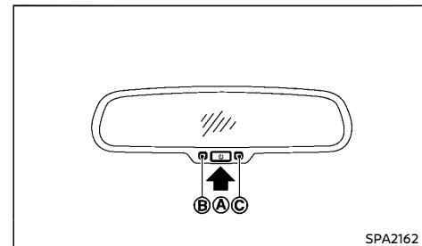
The inside rearview mirror is designed so that it automatically changes reflection according to the intensity of the headlights of the vehicle following you.
