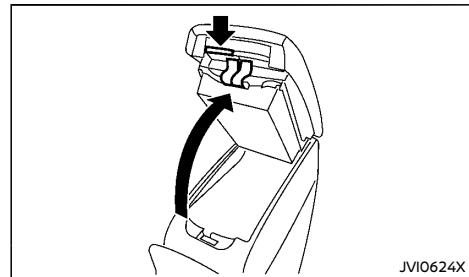
Pull up on the passenger's side latch to open the lower half of the console box. A power outlet is located inside the console box.
