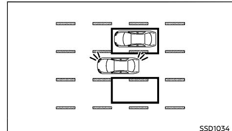
If the driver activates the turn signal while another vehicle is in the detection zone, then the Blind Spot Indicator light flashes and a chime will sound twice.
