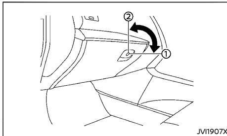
Open the glove box by pulling the handle. Use the mechanical key when locking ① or unlocking ② the glove box.
