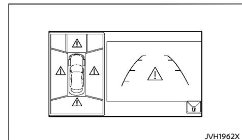
When the "!" icon is displayed on the screen, there will be abnormal conditions in the Intelligent Around View Monitor. This will not hinder normal driving operation but the system should be inspected by a NISSAN dealer.
