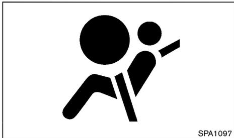
The SRS air bag warning light, displaying
