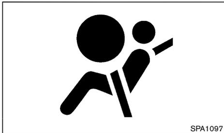
The SRS air bag warning light, displaying
