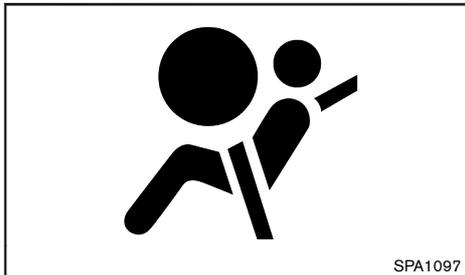
The supplemental air bag warning light, displaying
