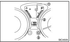
The odometer/twin trip odometer is displayed when the ignition switch is in the "ON" position.
