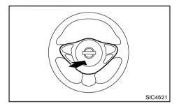
The horn switch operates regardless of the ignition switch position except when the battery is discharged. When the horn switch is pushed and held, the horn will sound. Releasing the horn switch will cease the horn sound.
