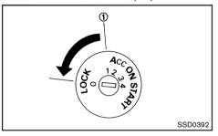
The ignition switch includes a device that helps prevent accidental removal of the key while driving.
