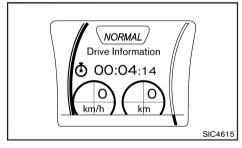
While in the Drive Mode, push the Drive information button to display elapsed time, average speed and trip distance. Pressing the Drive information button a second time or turn the Selection dial will display a G (gravity)-Force screen.
