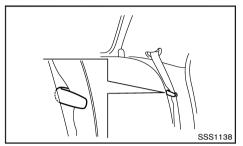
When the rear seat belts are not in use and when folding down the rear seats, hook the rear outer seat belts on the seat belt hooks.
