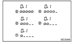
When the ignition switch is in the "ON" position, engine oil information is displayed on the vehicle information display in the following order:
