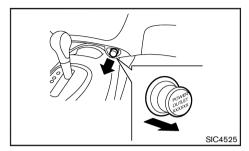
The power outlet is for powering electrical accessories.
