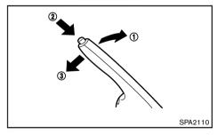
To apply the parking brake, pull the parking brake lever up  $\widehat{\mathbf{1}}$ .
