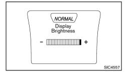
4. Turn the Selection dial to + to increase brightness or to - to decrease brightness, then press the Enter button to apply the selection.
