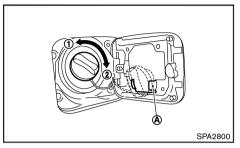
Except for Korea: The fuel filler cap is a ratcheting type. Turn the cap counterclockwise ① to remove. Tighten the cap clockwise ② until ratchet clicks, more than twice, after refueling.
