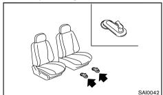
This vehicle includes front floor mat brackets to act as a floor mat positioning aid. NISSAN floor mats have been specially designed for your vehicle models.
