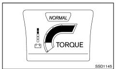
The NORMAL drive mode is recommended for normal driving. To set the NORMAL drive mode, press the drive mode select button and then press the NORMAL drive mode button. The control state of the engine, CVT (if equipped), STRG\* (if equipped) and climate is displayed briefly.
