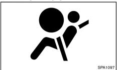
The supplemental air bag warning light, displaying in the instrument panel, monitors the circuits for the air bag systems, pre-tensioner seat belt systems and all related wiring.
