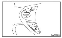
The control buttons for the Bluetooth<sup>®</sup> Hands- Free Phone System are located on the steering wheel.
