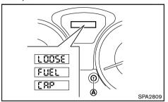
The LOOSE FUEL CAP warning message is displayed on the vehicle information display when the fuel-filler cap is not tightened correctly after the vehicle has been refueled. It may take a few driving trips for the message to be displayed. To turn off the warning message, do the following procedure:
