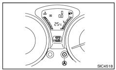
The switch for the trip computer is located on the meter panel.
