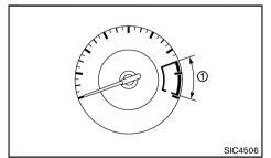
The tachometer indicates the engine speed in revolutions per minute (rpm). Do not rev the engine into the red zone (1).
