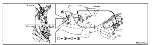
If the booster battery is in another vehicle (B), position the two vehicles (A) and (B) to bring the batteries into close proximity to each other.
