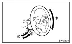
Push the lock lever down (1) and adjust the steering wheel up or down (2) to the desired position.
