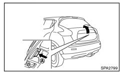
To open the back door, unlock it and push the back door opener switch (A). Pull up the back door to open.
