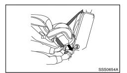
Step 2 Route the seat belt tongue through the child restraint and insert it into the buckle (2) until you
