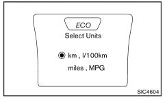
Turn the Selection dial to select "km, I/100km" or "miles, MPG", then press the Enter button to apply the selection.
