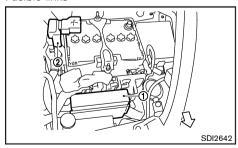
If any electrical equipment does not operate and the fuses are in good condition, check the fusible links in the holders (1) and (2). If any of these fusible links are melted, replace only with genuine NISSAN parts.
