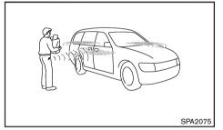
The Intelligent Key functions can only be used when the Intelligent Key is within the specified operating range from the request switch (1).
