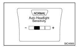
Turn the Selection dial to + to increase sensitivity or to - to decrease sensitivity, then press the Enter button to apply the selection.
