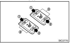
The seats can be warmed by built-in heaters. The switches located on the center console can be operated independently of each other.
