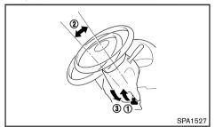
While pulling the lock lever up (1), adjust the steering wheel up or down (2) until the desired position is achieved.
