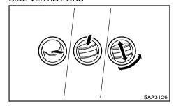
Open or close the vents, and adjust the air flow direction of ventilators as illustrated.
