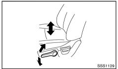
Pull up or push down the adjusting lever to adjust the seat height until the desired position is achieved.
