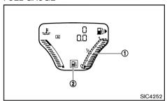
The fuel gauge ① indicates the approximate fuel level in the tank when the ignition switch is in the "ON" position.
