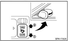
The outside rearview mirror remote control operates when the ignition switch is in the "ACC" or "ON" position.
