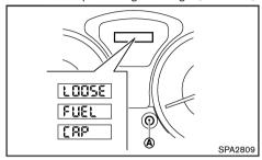
Push the reset switch (A) for more than 1 second to reset the LOOSE FUEL CAP warning message after the fuel cap has been tightened. For additional information see "Fuel filler cap" (P.3-17).
