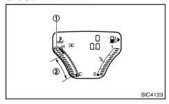
The engine coolant temperature gauge (1) indicates the engine coolant temperature.
