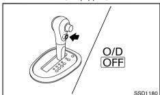
To select the overdrive "OFF" position, push the overdrive switch with the shift lever in the "D" (Drive) position. The overdrive indicator light OFF in the meter panel illuminates. To select the overdrive "ON" position, push the overdrive switch again. The overdrive indicator light will turn off. When the shift lever is shifted to any position other than "D", the overdrive will be automatically "ON" position.
