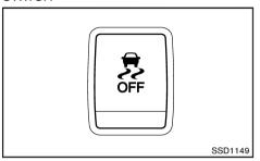
The vehicle should be driven with the Vehicle Dynamic Control (VDC) system ON for most driving conditions.
