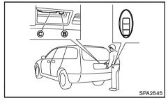
When you carry the Intelligent Key with you, you can lock or unlock all doors by pushing the door handle request switch (driver's or front passenger's) (A) or back door request switch (B) within the range of operation.
