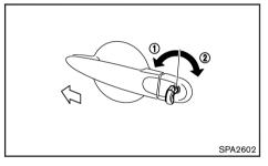
To lock the door, insert the key to the door key cylinder and turn the key to the front side of the vehicle 1. The driver's side door will lock.
