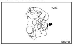
The engine serial number is stamped on the engine as shown.
