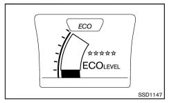
The ECO drive mode is recommended for maximum fuel economy. In the ECO drive mode, the engine and CVT (if equipped) are adjusted to enhance fuel economy.
