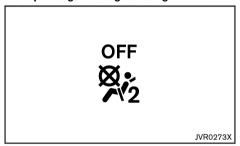
The front passenger air bag status light is located on the instrument panel. After the ignition switch is placed in the "ON" position, the front passenger air bag status light illuminates for about 7 seconds and then turns off or operates depending on the front passenger seat occupied status. The light operates as follows:
