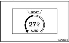
While the Climate mode is indicated on the display screen, the room temperature and fan speed, and automatic mode or manual mode, are indicated by the full screen. To indicate the climate mode, push the "CLIMATE" button.
