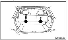
The anchor points are located on the back side of the seatbacks.
