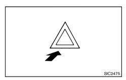
The hazard indicator flasher switch operates regardless of the ignition switch position except when the battery is discharged.
