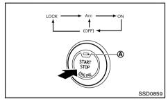
When the ignition switch is pushed without depressing the brake pedal (Continuously Variable Transmission models) or the clutch pedal (Manual Transmission models), the ignition switch position will change as follows:
