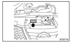
The air conditioner specification label is attached to the engine compartment as shown.
