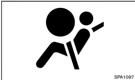
The supplemental air bag warning light, displaying
