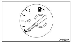
The fuel gauge indicates the approximate fuel level in the tank when the ignition switch is in the "ON" position.
