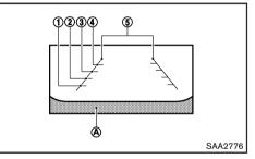
Guide lines which indicate the vehicle width and distances to objects with reference to the bumper line  $(\widehat{\mathbf{A}})$  are displayed on the monitor.
