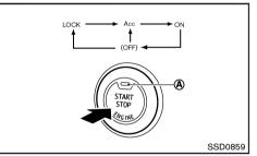
When the ignition switch is pushed without depressing the brake pedal, the ignition switch position will change as follows:
