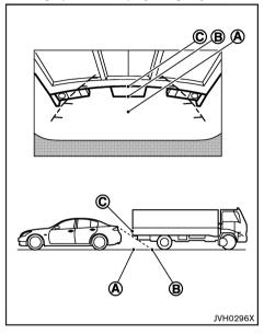
The position  $\bigcirc$  is shown further than the position B in the display. However, the position  $\bigcirc$  is actually at the same distance as the position A. The vehicle may hit the object when backing up to the position A if the object projects over the actual backing up course.
