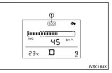
The ECO mode helps to enhance the fuel economy by controlling the engine and CVT operation automatically to avoid rapid acceleration.
