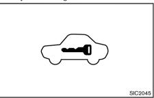
The security indicator light is located on the meter panel. It indicates the status of NATS.
