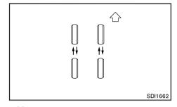
NISSAN recommends that tires be rotated every 10,000 km (6,000 miles). However, the timing for tire rotation may vary according to your driving habits and the road surface conditions. (For the tire replacement, see "Flat tire" (P.6-2).)
