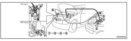
If the booster battery is in another vehicle (B), position the two vehicles (A) and (B) to bring the batteries into close proximity to each other.
