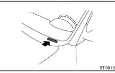
The vehicle identification number plate is attached as shown. This number is the identification for your vehicle and is used in the vehicle registration.
