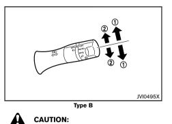
The turn signal switch will not be cancelled automatically if the steering wheel turning angle does not exceed the preset amount. After a turn or lane change, make sure that the turn signal switch is returned to its original position.
