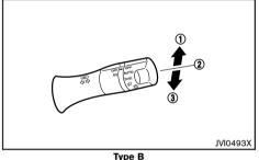
To turn on the high beam, push the lever towards the front position (1).
