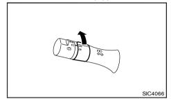
To turn on the rear fog light, turn the headlight switch to the  ${}_{\$} \bigcirc$  position, then turn the fog light switch to the  ${}_{\bigcirc} \ddagger$  position.
