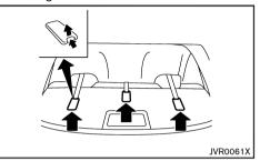
The anchor points are located on the rear parcel shelf for all three seating positions of the rear seat as shown (for Australia and New Zealand).
