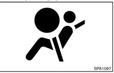
The supplemental air bag warning light, displaying tin the instrument panel, monitors the circuits for the air bag systems, pre-tensioners and all related wiring. When the ignition switch is in the "ON", the SRS air bag warning light illuminates for about 7 seconds and then turns off. This indicates that the SRS air bag systems are operational.
