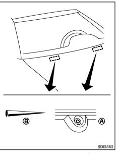
Be careful not to clog the washer nozzle (a) . This may cause improper windshield washer operation. If the nozzle is clogged, remove any objects with a needle or small pin (a) . Be careful not to damage the nozzle.
