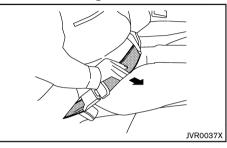
3. Position the lap belt portion low and snug on the hips as shown.
