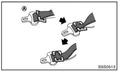
To prevent slack in the lap belt, it is necessary to secure the lap belt in place with a locking clip (A). Use the locking clip attached to the child restraint system, or one which is equivalent in dimensions and strength.
