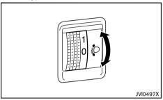
The headlight aiming control operates when the ignition switch is in the "ON" position and the headlight is on to allow the headlight axis to be adjusted according to the driving condition.
