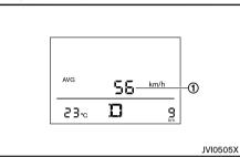
The average vehicle speed mode shows the average vehicle speed ① since the last reset. Resetting is done by pushing the D switch (A) for longer than 1 second. The display is updated every 30 seconds. The first 30 seconds after a reset, the display shows "——".
