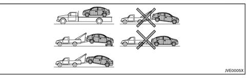
NISSAN recommends that towing dollies be used under the front wheels when towing your vehicle or the vehicle be placed on a flatbed tow truck as illustrated.
