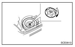
Remove the jack, necessary tools and the spare tire from the storage area.
