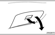
Type A To open the glove box, pull the handle. To close, push the lid in until the lock latches.
