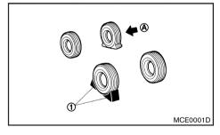
Be sure to block the appropriate wheel to prevent the vehicle from moving, which may cause personal injury.
