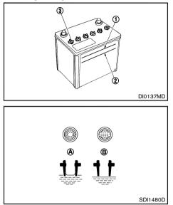
Check the fluid level in each cell. The battery fluid level should be between the UPPER LEVEL 1 and LOWER LEVEL 2 lines.
