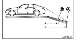
When backing up the vehicle down a hill, the distance guide lines and the vehicle width guide lines are shown further than the actual distance. For example, the display shows 1 m (3 ft) to the place (A), but the actual 1 m (3 ft) distance on the hill is the place (B). Note that any object on the hill is viewed in the monitor closer than it appears.
