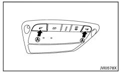
To turn the map light on, push the switch (A) as illustrated. To turn the light off, push the switch again.
