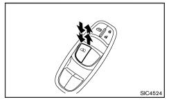
The automatic function is available for the switch that has an  $(\underline{A})$  mark on its surface.
