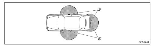
The Intelligent Key functions can only be used when the Intelligent Key is within the specified operating range from the request switch (1).
