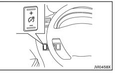
The instrument brightness control operates when the ignition switch is in the "ON" position.
