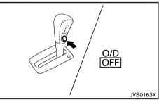
To select the overdrive "OFF" position, push the overdrive switch with the shift lever in the "D" (Drive) position. The overdrive indicator light  $OP \\ OFF$  in the meter panel illuminates. To select the overdrive "ON"
