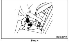
Remove any additional slack from the seat belt; 4. press downward (3) and rearward (4) firmly in the center of the child restraint with your knee to compress the vehicle seat cushion and seatback while pulling up on the seat belt.
