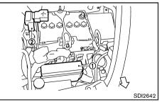
If any electrical equipment does not operate and the fuses are in good condition, check the fusible links in
