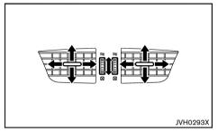
Open/close the ventilators by moving the control in either direction.
