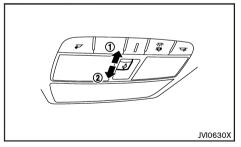
The sunroof operates when the ignition switch is in the "ON" position.
