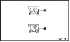
6. If the fuse is open  $\textcircled{\textbf{A}}$  , replace it with a new fuse  $\textcircled{\textbf{B}}$  .
