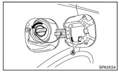
The fuel filler cap is a ratcheting type. Turn the cap counterclockwise to remove. Tighten the cap clockwise until ratchet clicks, more than twice, after refueling.
