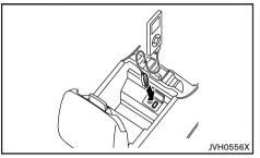
The USB outlet connector is located in the center console. Open the USB outlet connector lid and connect the iPod cable to the USB connector. The battery of the iPod is charged while the connection to the vehicle.
