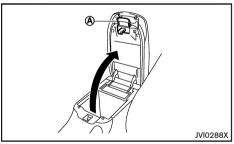
To open the console box lid, push the knob  $\textcircled{\sc and}$  and pull up the lid.
