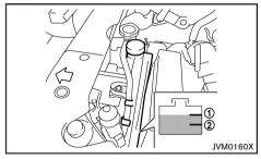
Check the coolant level in the reservoir tank when the engine is cold. If the coolant level is below the MIN level (2), add coolant up to the MAX level (1). If the reservoir tank is empty, check the coolant level in the radiator when the engine is cold. If there is insufficient coolant in the radiator, fill the radiator with coolant up to the filler opening and also add it to the reservoir tank up to the MAX level (1).
