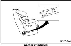
ISOFIX child restraints include two rigid attachments that can be connected to two anchors located in the seat. With this system, you do not have to use a vehicle seat belt to secure the child restraint. Check your child restraint for a label stating that it is compatible with the ISOFIX child restraints. This information may also be in the instructions provided by the child restraint manufacturer.
