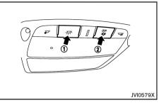
To turn on the map lights (both sides), push the switch (1). To turn off the lights, push the switch again.
