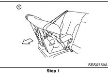
Be sure to follow the manufacturer's instructions for the proper use of your child restraint. Follow these steps to install a rear-facing child restraint on the rear seats using three-point type seat belt:
