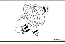
While pulling the lock lever up (1), adjust the steering wheel up, down, forward or rearward (2) until the desired position is achieved.
