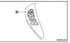
The switch for the trip computer is located on the left side of the steering wheel.
