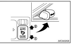
The outside rearview mirrors fold automatically by interlocking door lock. The function can be used while the switch is in the "AUTO" position (2).
