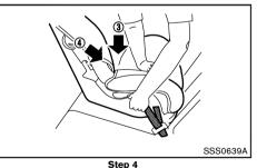
4. Remove any additional slack from the seat belt; press downward (3) and rearward (4) firmly in the center of the child restraint with your hand to compress the vehicle seat cushion and seatback while pulling up on the seat belt.
