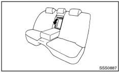
The rear center seatback can be folded to allow trunk access from inside the vehicle.
