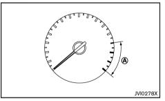
The tachometer indicates the engine speed in revolutions per minute (rpm). Do not rev the engine into the red zone (A) .
