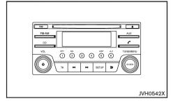
The audio system operates when the ignition switch is in the "ACC" or "ON" position.
