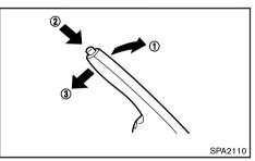
To apply the parking brake, pull the parking brake lever up  $(\mathbf{1})$ .
