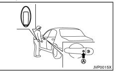
When you carry the Intelligent Key with you, you can lock or unlock all doors by pushing the door handle request switch (driver's or front passenger's) (A) within the range of operation.
