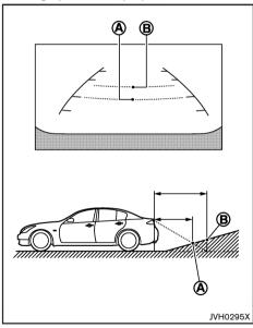
When backing up the vehicle up a hill, the distance guide lines and the vehicle width guide lines are shown closer than the actual distance. For example, the display shows 1 m (3 ft) to the place  $(\mathbf{A})$ , but the
