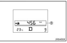
The distance to empty (dte) mode provides you with an estimation of the distance ① that can be driven before refueling. The dte is constantly being calculated, based on the amount of fuel in the fuel tank and
