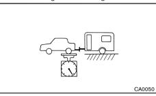
The rear gross axle weight must not exceed the Gross Axle Weight Rating (GAWR).
