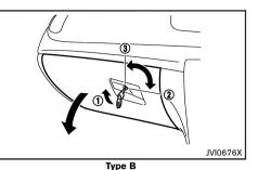
To open the glove box, pull the handle (1).
