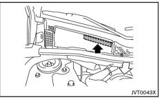
The vehicle identification number is located as shown. Remove the cover to access the number.
