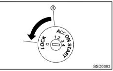
The ignition lock is designed so that the ignition switch cannot be turned to the "LOCK" position until the shift lever is moved to the "P" (Park) position. When moving the ignition switch to the "LOCK" position, to remove the key from the ignition switch, make sure the shift lever is in the "P" (Park) position.
