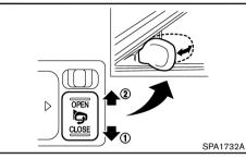
The outside rearview mirror remote control operates when the ignition switch is in the "ACC" or "ON" position.
