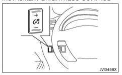
The instrument brightness control operates when the ignition switch is in the "ON" position.
