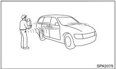
The Intelligent Key functions can only be used when the Intelligent Key is within the specified operating range from the request switch  $\widehat{(1)}$ .
