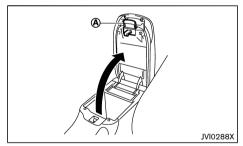
To open the console box lid, push the knob (A) and pull up the lid.
