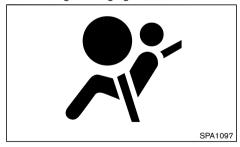
The SRS air bag warning light, displaying si in the instrument panel, monitors the circuits for the air bag systems, pre-tensioners and all related wiring.
