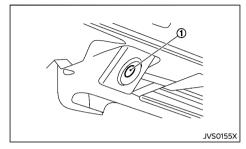
The rearview camera unit ① for the LDW/BSW systems is located above the rear license plate. To maintain the proper operation of the LDW/BSW systems and help keep the system functioning, be sure to observe the following:
