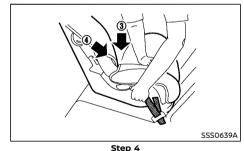
Remove any additional slack from the seat belt; press downward ③ and rearward ④ firmly in the center of the child restraint with your hand to compress the vehicle seat cushion and seatback while pulling up
