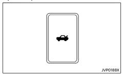
To open the trunk lid, push the opener switch for more than 1 second.
