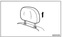
Make sure the head restraint is positioned from the stored position or any non-latch position so the lock knob is engaged in the notch before riding in that designated seating position.
