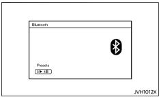
To switch to the Bluetooth® audio mode, push the USB AUX button repeatedly until the Bluetooth® audio mode is displayed on the screen.
