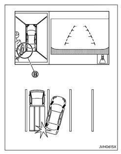
There may be a small distance visible between the vehicle and the object in the bird's-eye view on the display (B).
