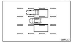
The Blind Spot Indicator light illuminates if you overtake a vehicle and that vehicle stays in the detection zone for approximately 3 seconds.
