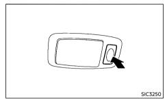
To turn the rear personal lights on, push the switch. To turn them off, push the switch again.
