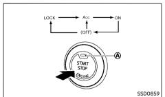
When the ignition switch is pushed without depressing the brake pedal, the ignition switch position will change as follows:
