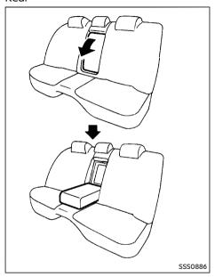
The rear center seatback can be folded to make the rear armrest. Fold down the seatback until it becomes horizontal.
