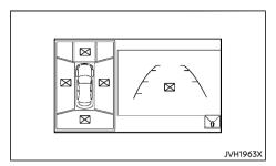
When the "[X]" icon is displayed on the screen, the camera image may be receiving temporary electronic disturbances from surrounding devices. This will not hinder normal driving operation but the system should be inspected by a NISSAN dealer if it occurs frequently.
