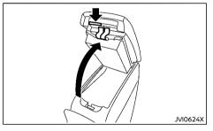
Pull up on the passenger's side latch to open the lower half of the console box. A power outlet is located inside the console box
