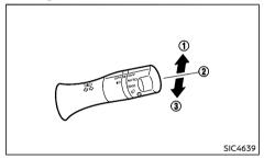
To turn on the high beam, push the lever towards the front position  $\widehat{\mathbb{Q}}$ .
