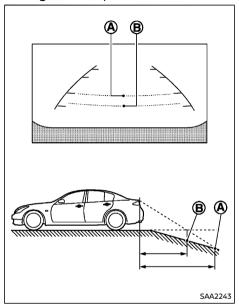
When moving the vehicle down a hill, the distance guide lines and the vehicle width guide lines are shown further than the actual distance. For example, the display shows 1 m (3 ft) to the place (a), but the actual 1 m (3 ft) distance on the hill is the place (b). Note that any object on the hill is viewed in the monitor closer than it appears.
