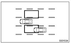
The Blind Spot Indicator light illuminates if a vehicle enters the detection zone from behind in an adjacent lane.
