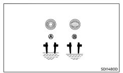
Check the fluid level in each cell. The battery fluid level should be between the UPPER LEVEL. and LOWER LEVEL (2) lines.
