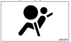
The supplemental air bag warning light, displaying in the instrument panel, monitors the circuits for the air bag systems, pretensioner seat belt systems and all related wirina.
