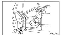
Warning labels about the supplemental air bag system are placed in the vehicle as shown in the illustration.
