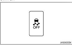
The vehicle should be driven with the Vehicle Dynamic Control (VDC) system on for most driving conditions.
