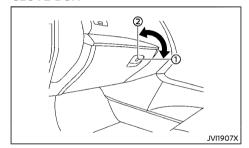
Open the glove box by pulling the handle. Use the mechanical key when locking (1) or unlocking (2) the glove box.
