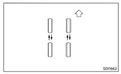
NISSAN recommends that tires be rotated every 10,000 km (6,000 miles). However, the timing for tire rotation may vary according to your driving habits and the road surface conditions. (See "Flat tire" (P.6-2) for the tire replacement.)
