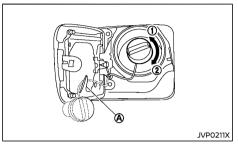
The fuel-filler cap is a ratcheting type. Turn the cap counterclockwise (1) to remove. Tighten the cap clockwise (2) until ratchet clicks, more than twice, after refueling.
