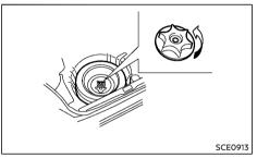
Remove the jack, necessary tools and the spare tire from the storage area located under the trunk.
