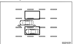
If the driver activates the turn signal, then the Blind Spot Indicator light flashes and a chime will sound twice.
