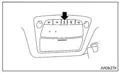
The console light will turn on whenever the clearance lights or headlights are illuminated.
