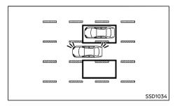
If the driver activates the turn signal while another vehicle is in the detection zone, then the Blind Spot Indicator light flashes and a chime will sound twice.
