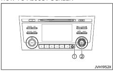
To set up the rear view monitor to your preferred settings, push the ENTER/SETTING button (2) while the rear view monitor screen is displayed. Each time the ENTER/SETTING button (2) is pushed, the next setting item is selected. Turn the TUNE-FOLDER control knob. 1) to adjust each item.
