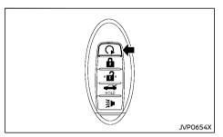
The remote engine start  $\Omega$  button is on the Intelligent Key if the vehicle has remote engine start function. This function allows the engine to start from outside the vehicle.
