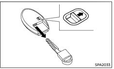
To remove the mechanical key, release the lock knob at the back of the Intelligent Key.
