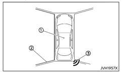
The bird's-eye view shows the overhead view of the vehicle which helps confirm the vehicle position and the predicted course to a parking space.
