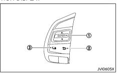
The vehicle information display can be changed using the switches
