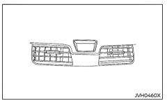
Adjust the air flow direction of the ventilators by moving the center knob (up/down, left/ right) until the desired position is achieved.
