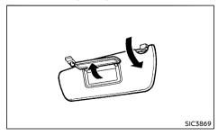
To access the vanity mirror, pull the sun visor down and flip open the mirror cover. Some vanity mirrors are illuminated and turn on when the mirror cover is open.
