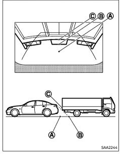
The position (C) is shown further than the position (B) in the display. However, the position © is actually at the same distance as the position (A). The vehicle may hit the object when moving toward the position (A) if the object projects over the actual moving course.
