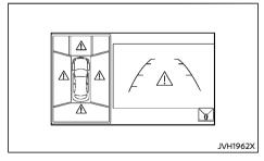
When the "!" icon is displayed on the screen, there will be abnormal conditions in the Intelligent Around View Monitor. This will not hinder normal driving operation but the system should be inspected by a NISSAN dealer.
