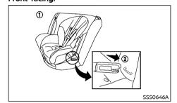
Front-facing: Steps 1 and 2 Be sure to follow the manufacturer's instructions for the proper use of your child restraint. Follow these steps to install a front-facing child restraint on the rear outboard seats using ISOFIX:
