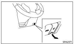
The fuel-filler lid release is located below the instrument panel. To open the fuel-filler lid, pull the release. To lock, close the fuel-filler lid securely.
