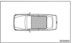
The Intelligent Key functions can only be used for starting the engine when the Intelligent Key is within the specified operating range as illustrated.
