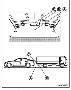
The position © is shown further than the position ® in the display. However, the position © is actually at the same distance as the position ⓐ. The vehicle may hit the object when backing up to the position ⓐ if the object projects over the actual backing up course.
