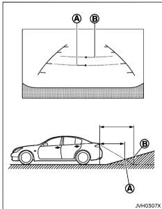
When moving the vehicle up a hill, the distance guide lines and the vehicle width guide lines are shown closer than the actual distance. For example, the display shows 1 m (3 ft) to the place A, but the actual 1 m (3 ft) distance on the hill is the place B. Note that any object on the hill is viewed in the monitor further than it appears.
