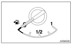
The fuel gauge indicates the approximate fuel level in the tank when the ignition switch is in the "ON" position.
