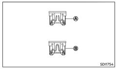
5. If the fuse is open (A), replace it with a new fuse (B).
