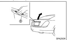
The trunk lid can be opened by pushing the trunk open request switch (1) when the Intelligent Key is within the operating range of the trunk lock/unlock function. (See "Intelligent Key system" (P.3-5).)
