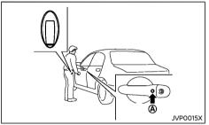
When you carry the Intelligent Key with you, you can lock or unlock all doors by pushing the door handle request switch (A) within the range of operation.
