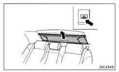
The rear sunshade operates when the ignition switch is in the "ON" position.
