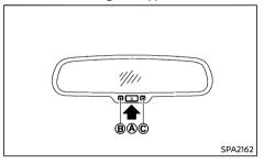
The inside rearview mirror is designed so that it automatically changes reflection according to the intensity of the headlights of the vehicle following vou.
