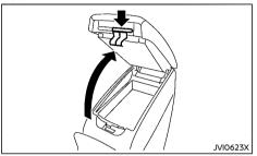
Pull up on the driver's side latch to open the upper half of the console box.
