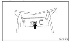
The AUX input jack is located on the center console. Open the lid and connect an audio device.
