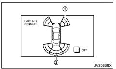
When the corner of the vehicle moves closer to an object, the corner sensor indicators ① appears.
