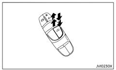
The automatic function is available for the switch that has an  $\boxed{\textbf{A}}$  mark on its surface.
