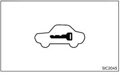
The security indicator light, located on the meter panel, operates whenever the ignition switch is in the "LOCK", "OFF" or "ACC" position. This is normal
