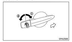
To lock the door, insert the mechanical key to the door key cylinder and turn the key to the front side of the vehicle (1). The driver's side door will lock.
