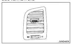
Open/close the ventilators by moving the control to either direction
