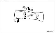
The rain-sensing auto wiper system can automatically turn on the wipers and adjust the wiper speed depending on the rainfall and the vehicle speed by using the rain sensor located on the upper part of the windshield.
