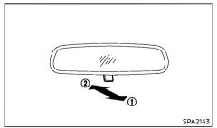
Pull the adjusting lever (1) when the glare from
