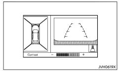
To set up the Intelligent Around View Monitor to your preferred settings, push the ENTER/ SETTING button ① while the Intelligent Around View Monitor screen is displayed. Each time the ENTER/SETTING button ① is pushed, the next setting item is selected. Turn the TUNE-FOLDER control knob ② to adjust each item.
