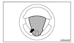
The horn switch operates regardless of the ignition switch position except when the battery is discharged.
