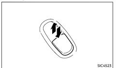
The passenger's switch can control its corresponding window.
