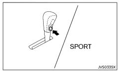
To select the SPORT mode, push the SPORT mode switch with the shift lever in the "D" (Drive) position. The SPORT mode indicator light sport in the meter panel illuminates. To turn off the SPORT mode, push the SPORT mode switch again. The SPORT mode indicator light will turn off. When the shift lever is shifted to any position other than "D" or "Ds", the SPORT mode will be automatically turned off.
