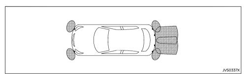
The parking sensor system sounds a tone to inform the driver of obstacles near the bumper. When the "Display" key is ON, the sensor view will automatically appear in the vehicle information display.
