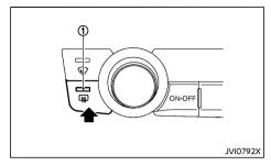
The defogger switch operates when the ignition switch is in the "ON" position.
