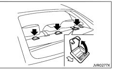
The anchor points are located under the anchorage cover on the rear parcel shelf finisher
