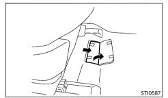
The vehicle identification number is stamped under the front right-side seat as shown.
