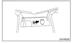
The USB connection port is located on the center console. Open the lid and connect a USB device or an iPod.
