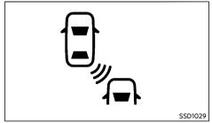
BSW indicator (in the vehicle information display) The BSW system operates above approximately 32 km/h (20 MPH).
