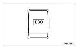
The ECO mode system helps to enhance the fuel economy by controlling the engine and CVT operation automatically to avoid rapid acceleration
