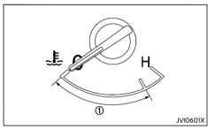
The engine coolant temperature gauge indicates the engine coolant temperature.
