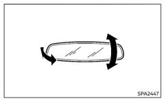
While holding the inside rearview mirror, adjust the mirror angles until the desired position is achieved
