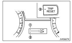
The odometer ① and the twin trip odometer ② are displayed below the vehicle information display when the ignition switch is placed in the "ON" position.
