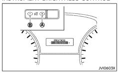
Push the "+" side (A) to increase the brightness of meter panel lights.
