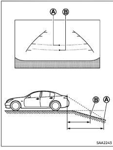
When moving the vehicle down a hill, the distance guide lines and the vehicle width guide lines are shown further than the actual distance. For example, the display shows 1 m (3 ft) to the place (a), but the actual 1 m (3 ft) distance on the hill is the place (b). Note that any object on the hill is viewed in the monitor closer than it appears.
