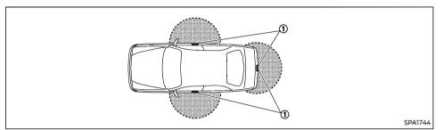
The Intelligent Key functions can only be used when the Intelligent Kev is within the specified operating range from the request switch (1).
