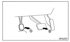
To apply the parking brake, firmly depress the parking brake pedal (1).
