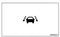
**LDW indicator (in the Vehicle information display)**The LDW system operates above approximately 70 km/h (45 MPH).
