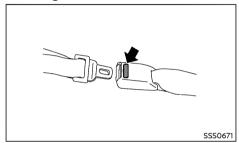
The center seat belt buckle is identified by the CENTER mark. The center seat belt tongue can be fastened only into the center seat belt buckle
